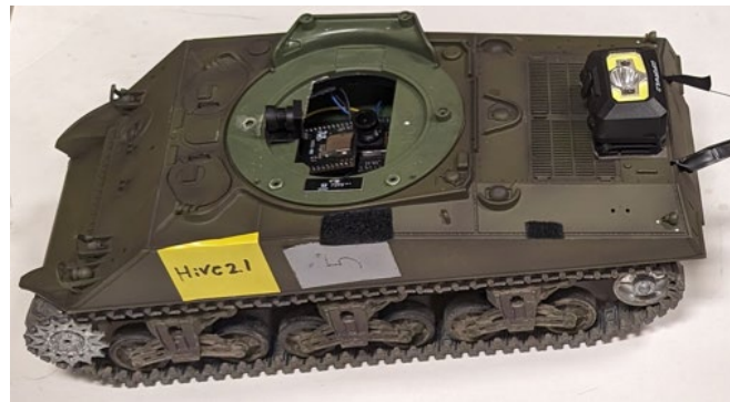
HIVE 2.1 Culvert inspection robot built with low-cost components and with simple design that allows for easy fabrication and maintenance
