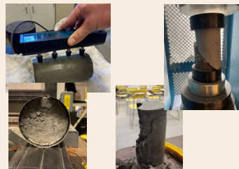
Figure 3. Select Laboratory Tests (Clockwise from top left: surface resistivity, slant shear bond, compressive strength and freeze-thaw conditioning tests)
