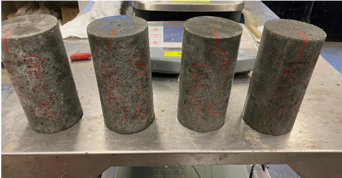
Figure 4-10: Mix Iteration PCC-2d Compressive Strength Specimens Before Conditioning
