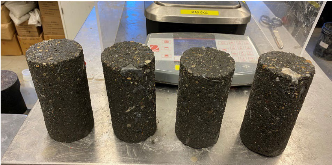
Figure 4-10: Mix Iteration PCC-2d Compressive Strength Specimens Before Conditioning
