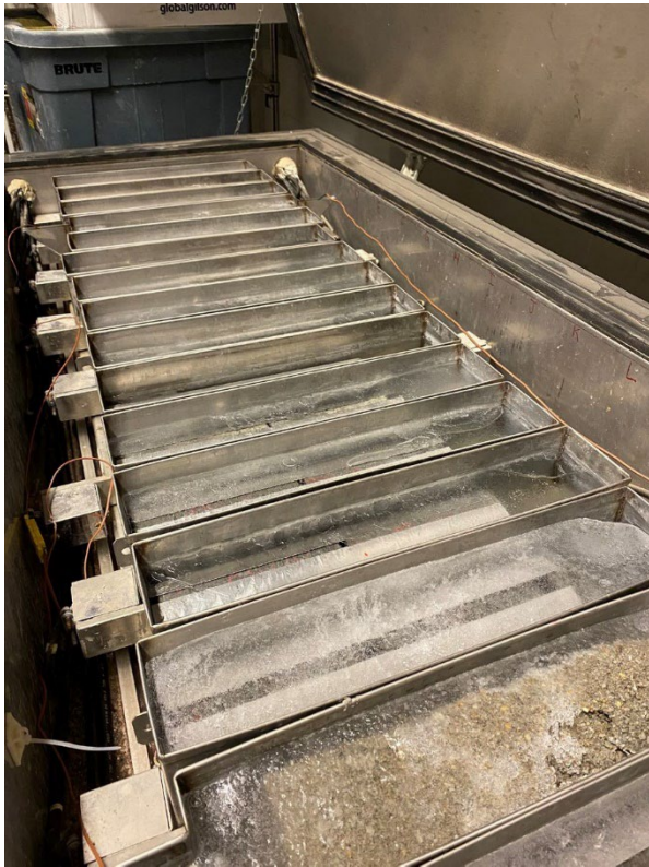
Figure 3-9: Stainless Steel Mold for Freeze Thaw Conditioning Chamber Placed Inside Freeze Thaw Chamber
