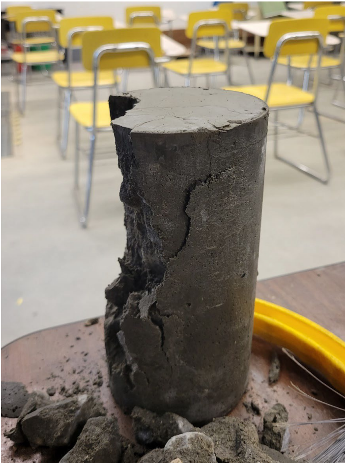
Figure 3-5: Compressive Strength Test Specimen After Failure
