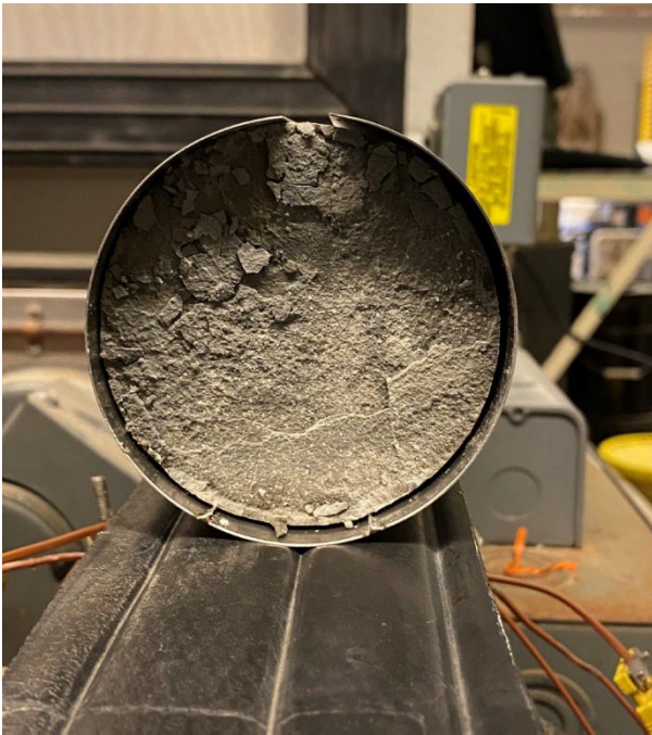
Figure 3-7: Stainless Steel Mold for Freeze Thaw Conditioning Chamber
