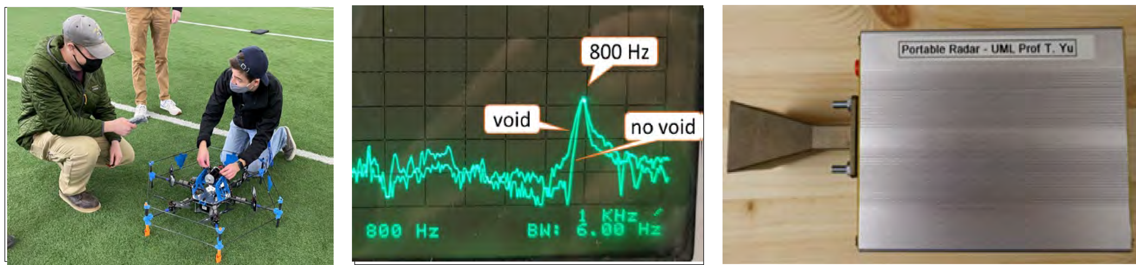
Figure 2. Custom UAV as AAS technology platform (left), Frequency spectrum analysis of known void (center), Compact 10 GHz microwave radar sensor (right)
