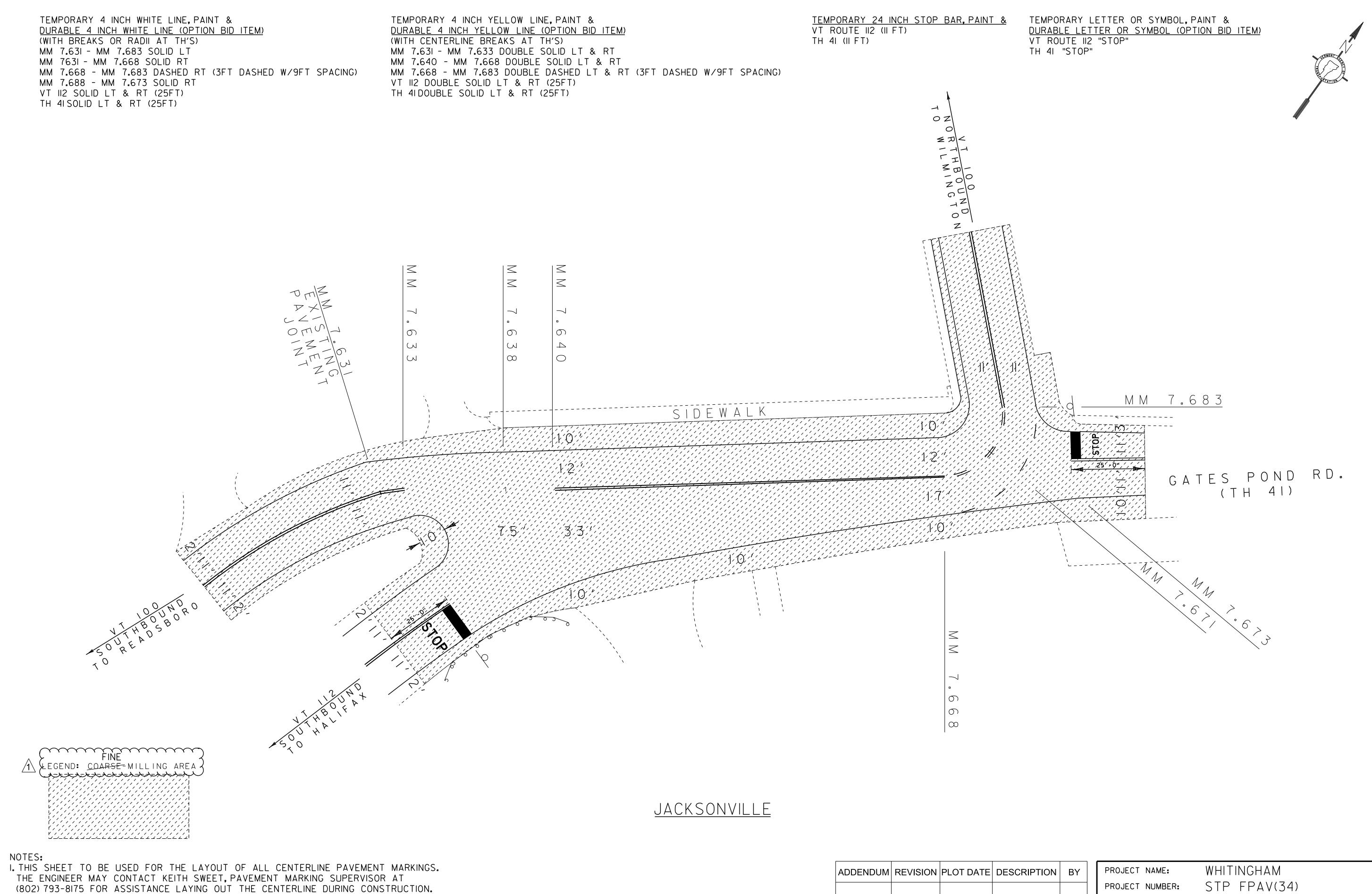
2. SEE PAVEMENT MARKING SHEETS FOR ADDITIONAL PAVEMENT MARKINGS. ONLY MARKINGS WITHIN THE MILLED AREA SHALL BE REPLACED OR AS DIRECTED BY THE ENGINEER.
