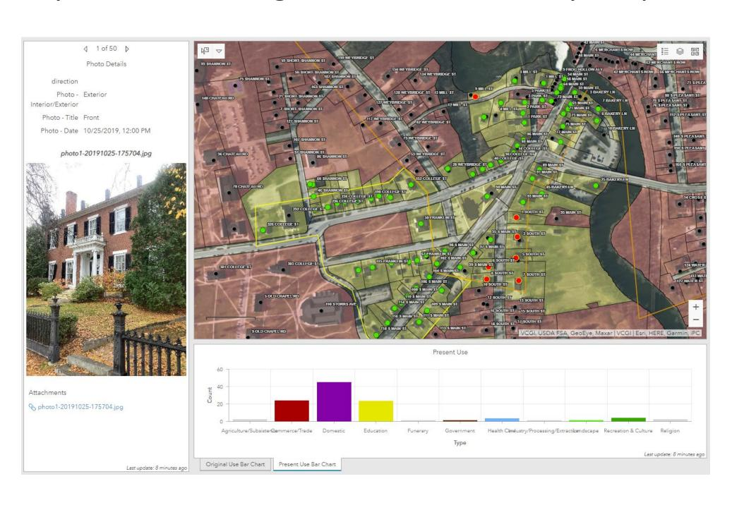
The Survey 123 interface for the VHSSS Form (left) and a view of the web map dashboard, which can display photographs and summary statistics for the survey area.
