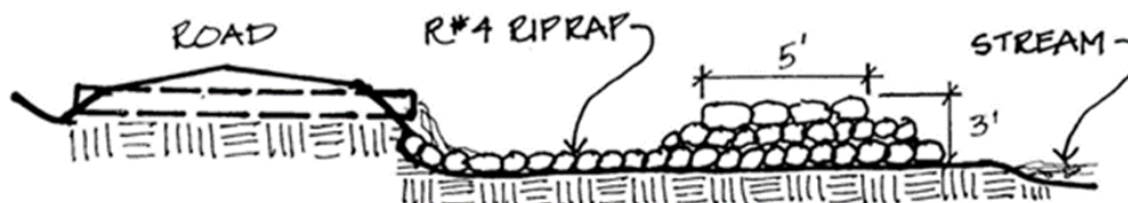
Figure 32: Plunge Pool – Section A-A View
