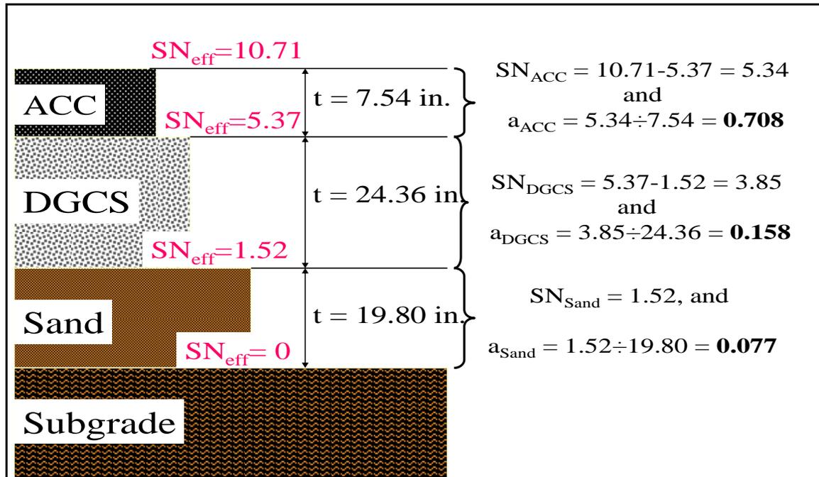
**Figure 5 – Determination of Layer Coefficients from FWD Testing**
