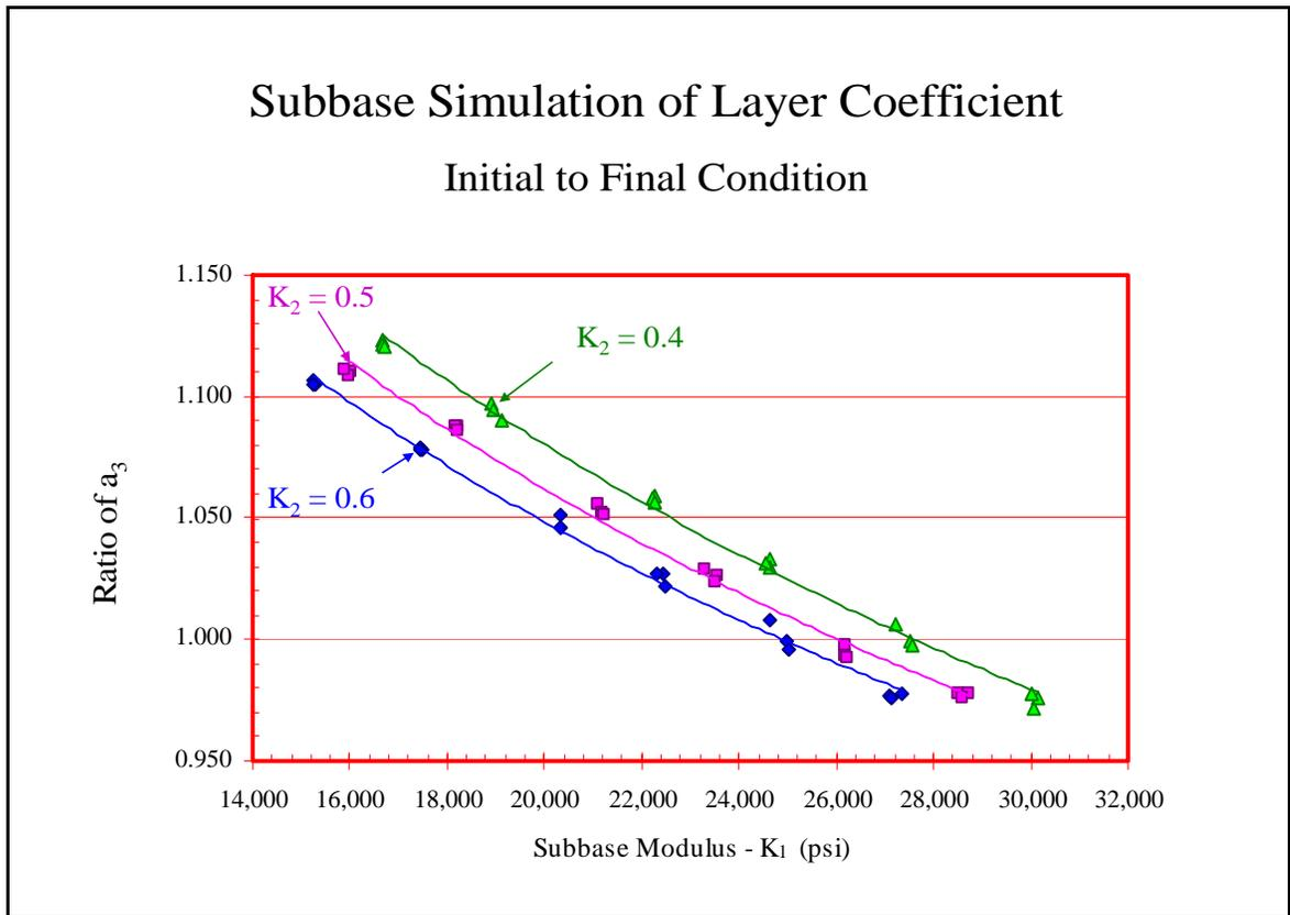
**Figure 3 – Subbase Simulation of Layer Coefficient**
