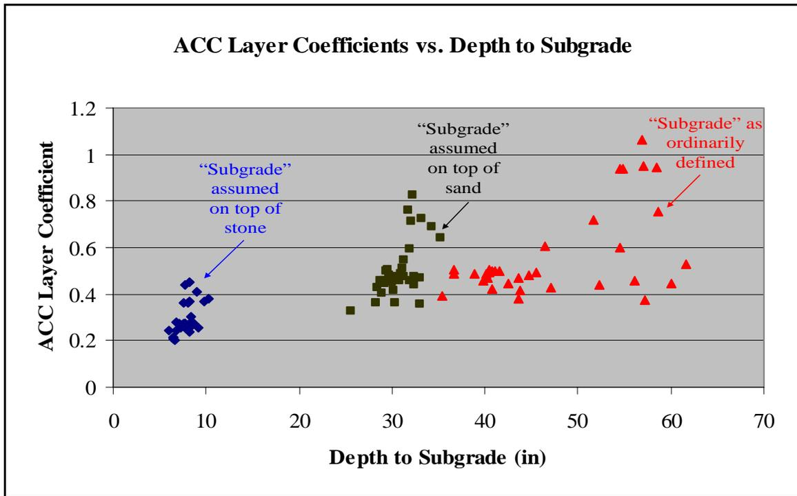
Figure 6 – ACC Layer Coefficient vs. Depth to Subgrade
