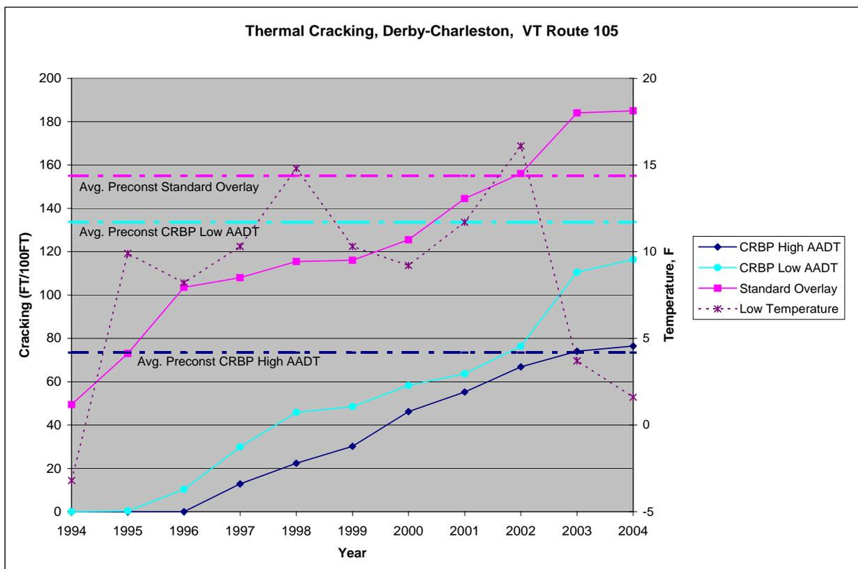
Figure 2 - Thermal Cracking
