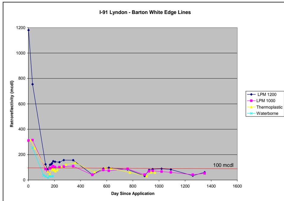
Figure 3 – Retroreflectivity Graph of White Edge Lines
