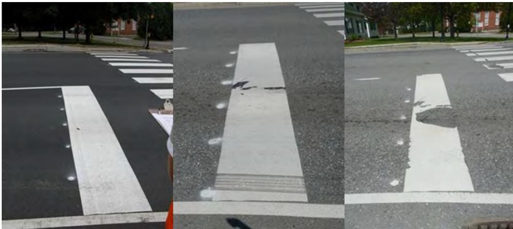
**Figure 4. Progressive wear characteristics of test site 3, from left to right, at 0, 8, and 19 months post construction.**
