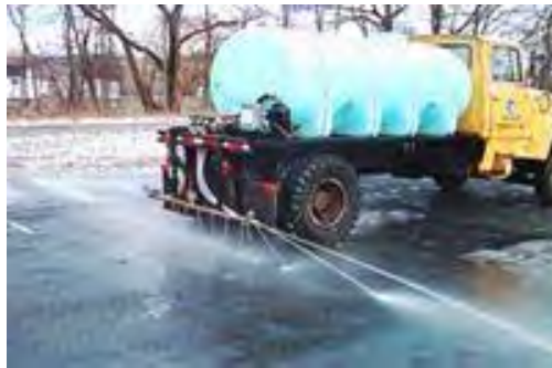
District 5's Tanker and Spray-bar system
