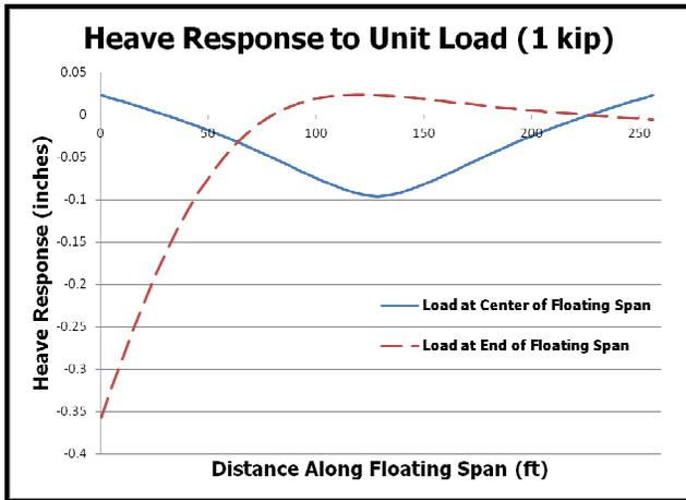
**Figure 8: Heave response to unit load.**
