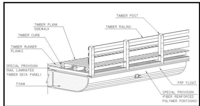
**Figure 3: FRP pontoon with timber decking, sidewalk, and railing.**
