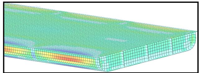
**Figure 7: Finite element model showing exterior plate stresses due to ice loading.**
