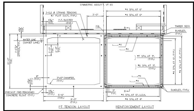
**Figure 2: Concrete pontoon alternative.**
