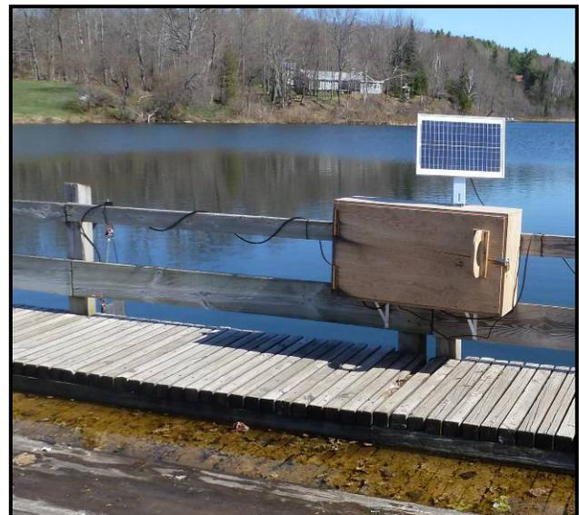
**Figure 4: Ice pressure monitoring equipment.**
