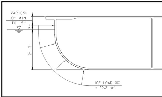
**Figure 6: Curved pontoon edges with ice load application.**
