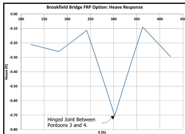
**Figure 5: Heave Response for hinged pontoon connection investigation.**
