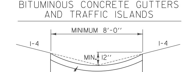
2" BITUMINOUS CONCRETE APPLIED
