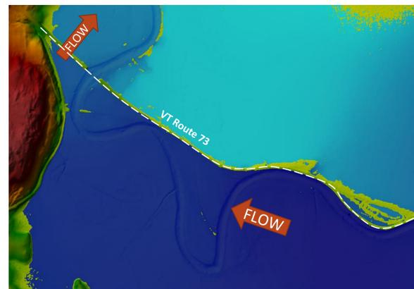
Figure 2. Backwaters can extend far upstream. Here, Rt. 73 increases WSE at 2 upstream bridges, 3.75 and 5.25 mi away, by 0.3 and 0.5ft, respectively. This can be alleviated by an increased bridge span or relief structures. The road grade can then be raised to eliminate overtopping.
