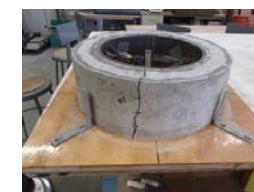
Figure 4. Confined shrinkage ring testing
