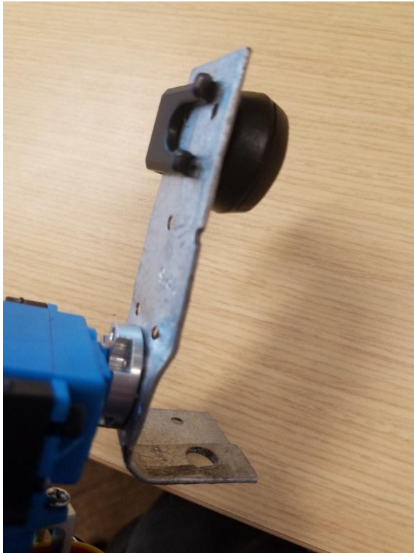
Figure 7 Showing New Mounting Bracket Developed by VTrans for Additional Lighting
