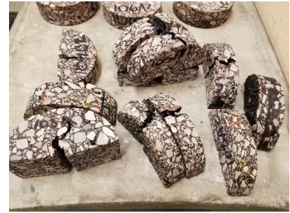
Left: HWTT specimens before & after testing. Right: I-FIT specimens post-testing
