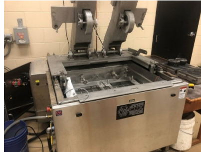
Left: HWTT equipment in Hot-mix lab. Right: I-FIT equipment with specimen loaded for testing
