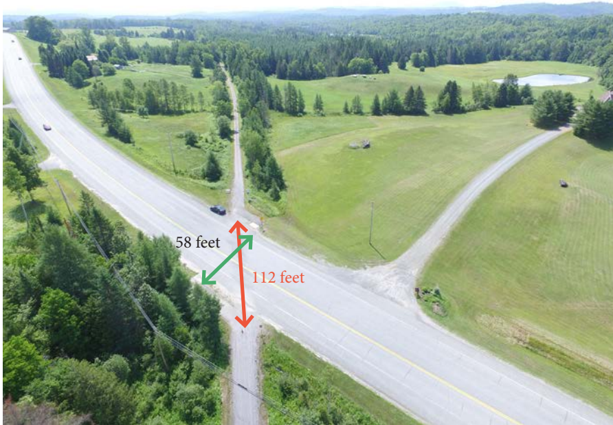
Crossing distances when crossing perpendicular to the road versus along the diagonal of the trail alignment
