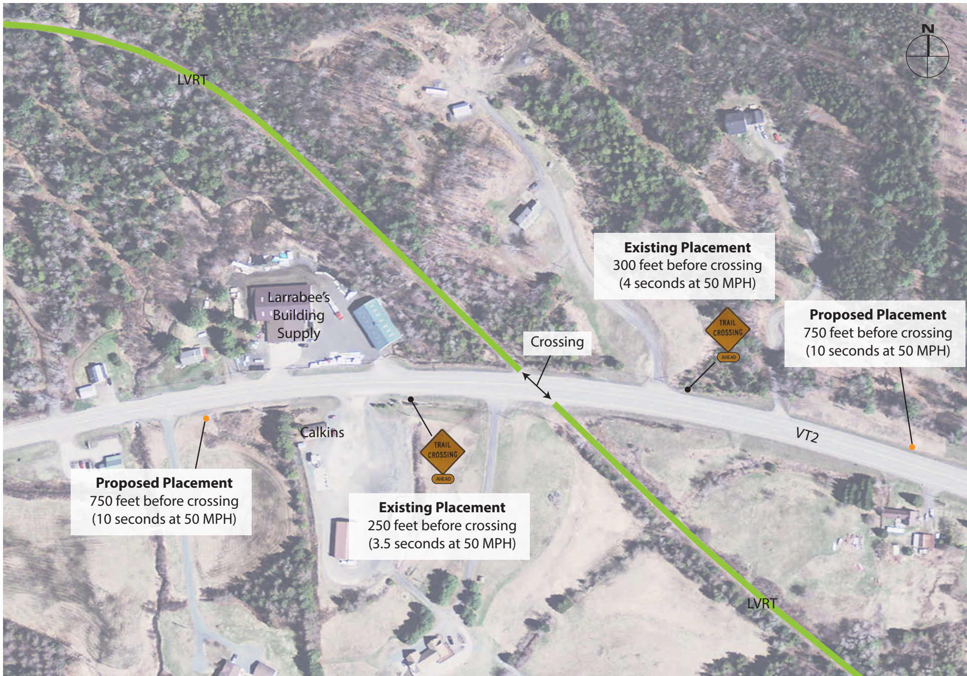
Figure 21. Existing and proposed advanced warning signs for the LVRT crossing of Route 2 near Larrabee's Building Supply
