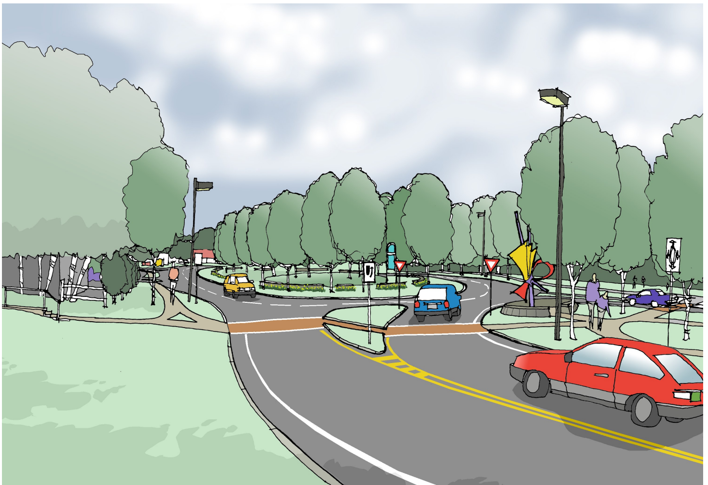
Sketch of the intersection after Alternative F improvements: Whereas a signalized intersection focuses on the enhancement of the roadside areas and the roadway itself remains as a large open paved area, the roundabout alternative redefines the street and intersection such that a landscape with integrity and identity is formed. The enhancement is of the whole roadway. Street trees, improved pedestrian crosswalks are all a part of the roundabout design, and similar to the previous design, a mini-park at the northern end is developed. Both plans intergate the traditional "Hairpin" sign for the Burlington Wayfinding system.
