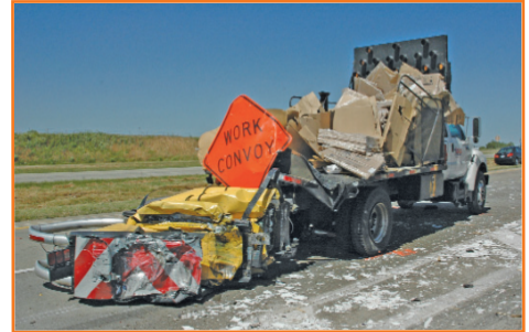
Truck-mounted attenuators before and after a vehicle impact (TTI).
