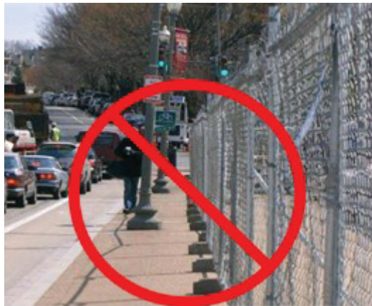
Figure 11. Diversion paths should be at least 60 inches wide to allow two wheelchairs to pass each other side-by-side (Sources: J. Barlow, Accessible Design for the Blind )
