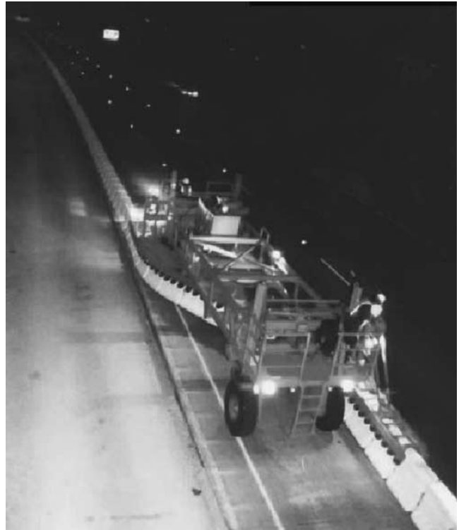
Figure 19. Proprietary portable barrier system, which can be shifted laterally by machine.
