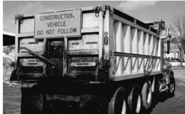
Figure 26. Reflectorized sign on the rear of haul truck.
