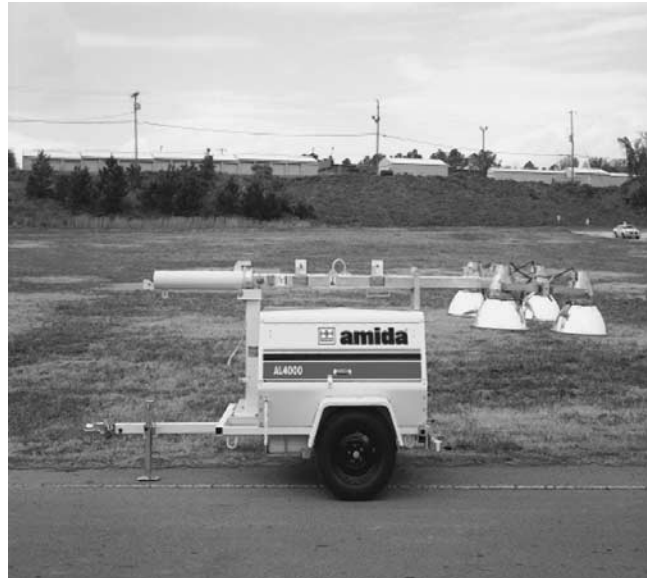
Figure 31. Portable trailer-mounted light tower being transported throughout the project.
