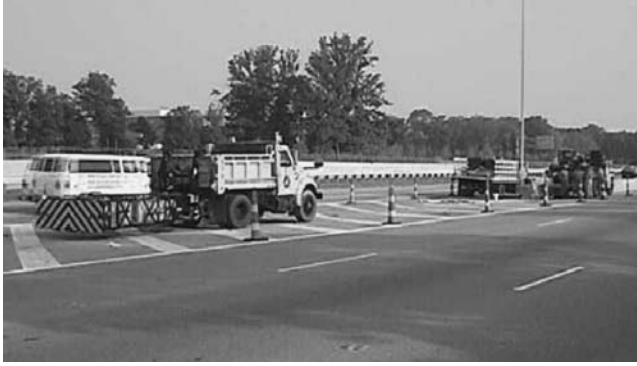
Figure 23. Shadow vehicle with truck-mounted attenuator.
