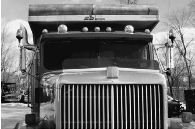
Figure 25. Warning lights mounted on the front of haul truck.
