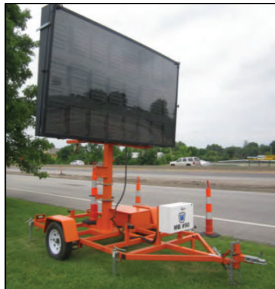
Figure 9 – Trailer-mounted PCMS (Source: Matt Myers, SAIC)
