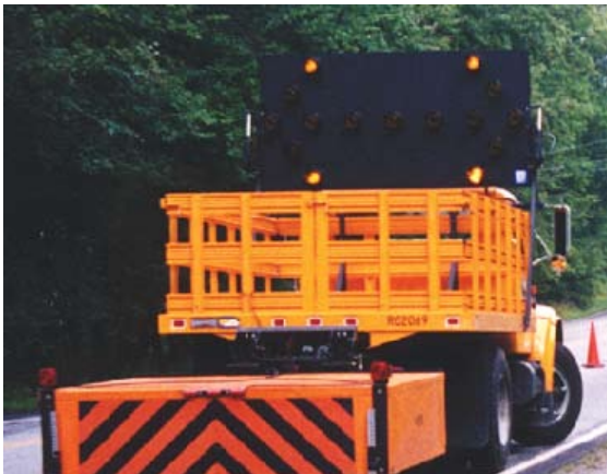
Figure 4. Shadow Vehicle with Attenuator
